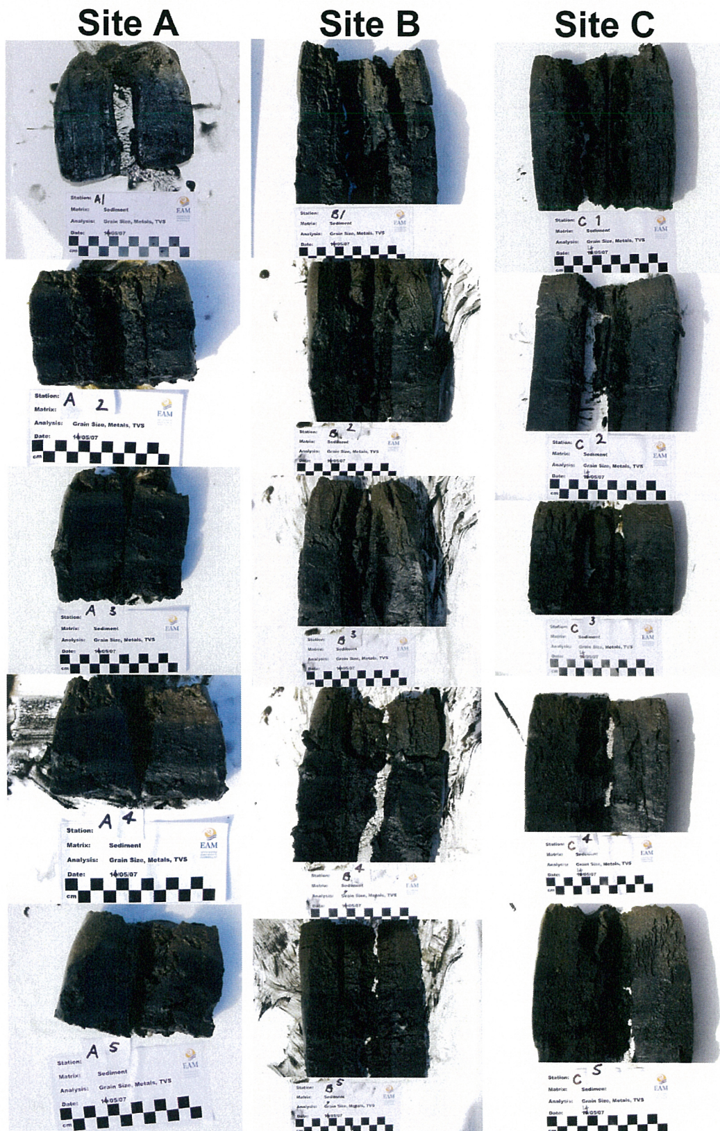
Figure 3: Sediment core profiles showing RPD and anoxic layers. Scale bar divisions = 1 cm
