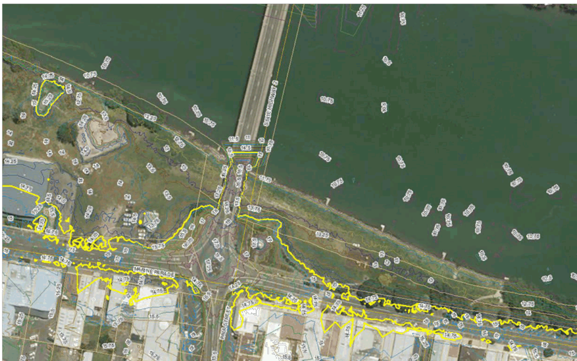
Image 3 – Contours adjacent to the bridge. The yellow contour is RL14.75m.
